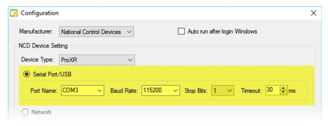
Select Port Name and Baud Rate. Keep default value for Stop Bits and Timeout.
