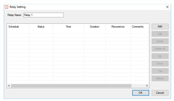
Relay Name: The relay can be given a name. It will be shown on the relay control panel. Schedule: The relay will be turned on/ off according to this schedule list.
