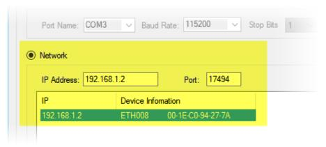
IP Address and Port number need to be input here.
